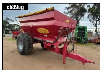
cb39ug BREDAL K85 8t cap/36m, trailing spreader. twin hydraulic driven spinners. Hopper cover . . . . . $77,000
