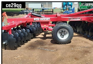
ce29gg 2024 SERAFIN ECO 24-26, 24 plate trailing disc harrows, 26" x 6 mm scalloped discs, oil bath bearings 230 mm spacing 150mm x 100mm $17,900
