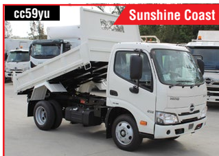
cc59yu Sunshine Coast 2024 HINO 300 616 at 2525 Tipper, 150hp, 47km, all steel, underbody hoist, auto release t/gate, drop sides/tail, #30480 $POA
