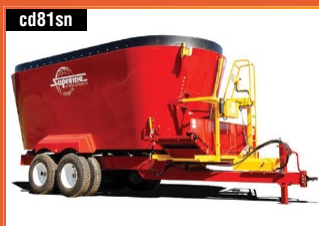
cd81sn 2024 SUPREME INTL 1500TR Supreme 1500T Tandem Axle, Triple Auger The 1500TR Pull-Type has a maximum payload of 50,000*
