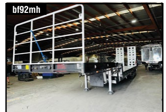
bf92mh BRAND NEW STONESTAR DECK WIDENER Drop Deck 45ft, Container Pins, 2pk paint finished, lots of tie points. . . $84,000+gst
