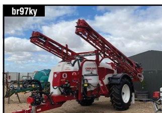
br97ky NEW 2023 CROPLANDS PINTO 4000 Stk# S30, 4,000L cpty, 24 mtr hydraulic lift & fold + wing tilt. Auto rate controller . $POA
