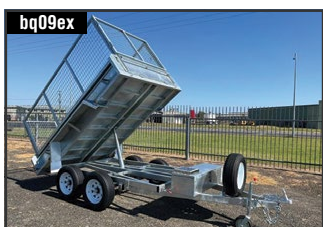
bq09ex 2022 MOORE 10'x5' 5 Stage Hydr Tipper Ram w/ 4T Loading Cap, 450mm Extra High Trailer Sides $8,409+GST
