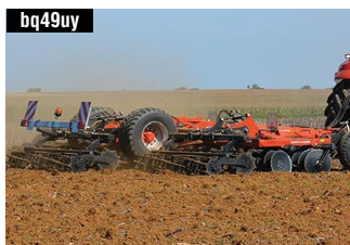
bq49uy GREGOIRE-BESSON NORMANDIE T70 900cm, 9 m width, 7,270 kg, Versatile machine for fast stubble cultivation.
