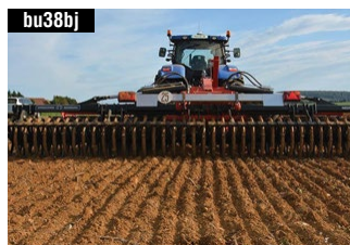
bu38bj GREGOIRE-BESSON NORMANDIE T60 600 cm, 6 m width, 4,820 kg, Versatile machine for fast stubble cultivation.
