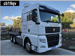
cb19qv 2024 SINOTRUK SITRAK C7H 540 HP, 12 Spd TraXon Trans, 8 Bag Air Ride, 90t GCM, EBS, ESC, EBL & ASR..... $POA
