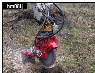
bm08lj FSI H65 STUMP GRINDER 12-20T, Hydr driven, 720mm dia wheel w/ 28 teeth, Oil 100-200l/min opt. .. $20,973
