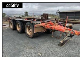
cd58fv 2011 JAMIESON DOLLY Triaxle Dolly, 10'1" Spread Airbag Suspension, Holland 50mm Turntable . . $22,727+GST
