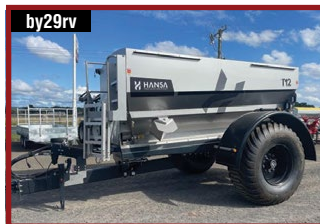
NEW 2023 HANSA T12 Stk# 100237, 11m3 capacity fertiliser spreader, 760mm chaff conveyor, 3m hydr braked axle... $POA
