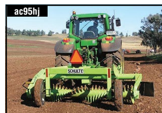
SCHULTE SRW1000 Rock Windrower is Designed to Windrow Small to Medium Rocks with Ease. $44,500
