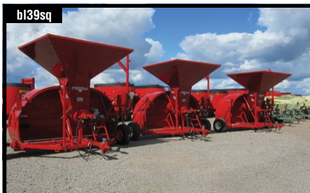
bl39sq NEW RENN RGB1020C Grain Bagger with 10ft wide tunnel & 20" auger. Unloader systems also available . . . . . $POA
