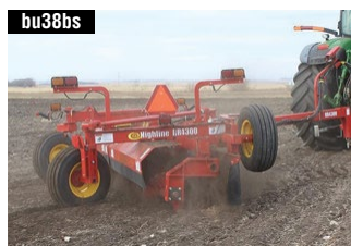
bu38bs HIGHLINE RR4300 180 cm, 430 cm, 4 m width, 1,806 kg, Rake rocks into narrow rows prior to picking.
