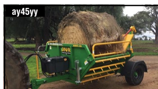
JNR BALE BULL BBR ROUND Two bales capacity, feed on both sides, made with heavy gauge steel full floor, all points are greaseable. . . . $20,500 + GST
