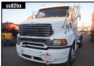
cc82bx 2003 STERLING AT9500 Detroit s-60 14lt engine, Rtlo-20918 gearbox, Meritor 46-160 diffs Airliner 90t susp . . . . Stk# 2630
