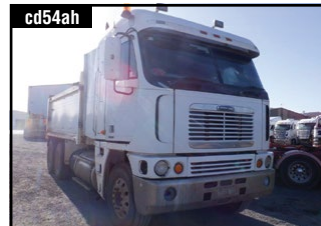
cd54ah 2003 FREIGHTLINER ARGOSY steel tipper, cat c15 eng, rtlo20918 g/box 46-160 meritor diffs, airliner susp. . . . . Stk# 2631
