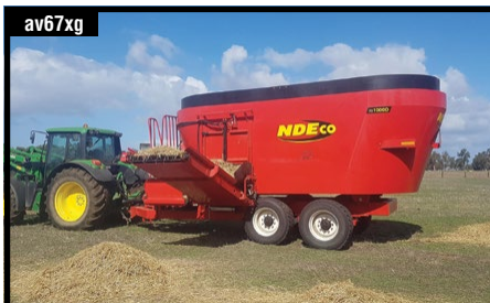
av67xg NDE FS1000D FS1000D Feedmixer with twin vertical augers, PTO drive, 28.4 cubic metres. Side elevator . . . . . $POA
