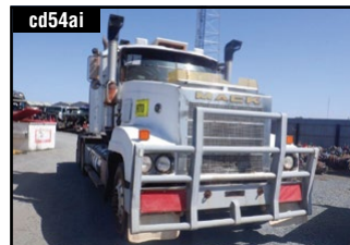
cd54ai 2003 MACK CLR caterpillar c-16 engine eaton 18spd gearbox mack diffs on neway suspension. . . . . Stk# 2636
