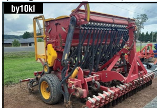
by10kl DUNCAN RENOVATOR MK4 382 cm, 3 m width, 2,030 kg, direct drill trailing, fixed frame, 25mm coil tynes fitted with Duncan T boot over $60,000
