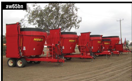
aw65bn NDE FS700 New 20 cubic metre Vertical Feedmixer. Single auger with 9 carbide-insert knives. Weightronix scales . . . . . $POA
